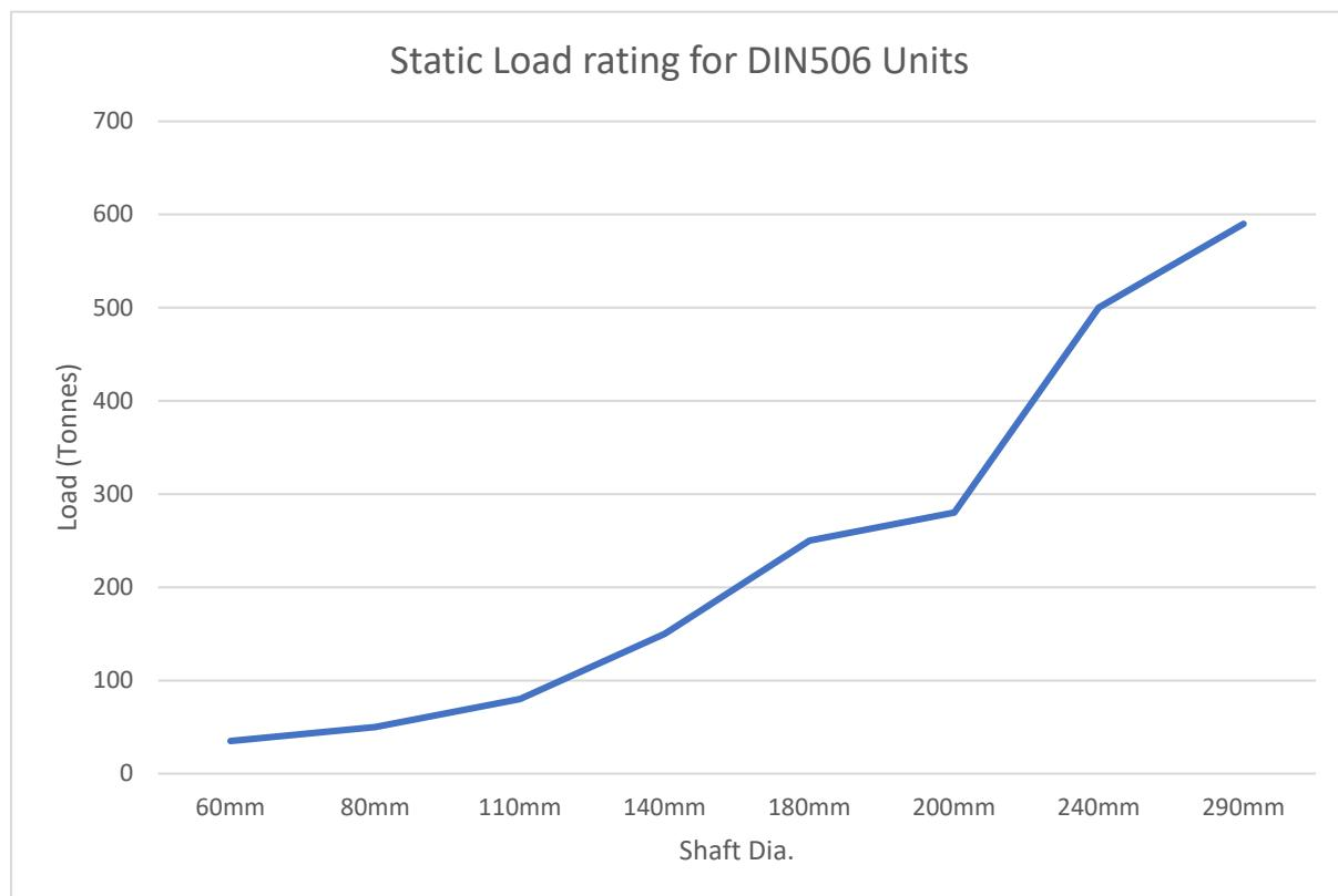
***The chart shown above details the static load capacity of DIN506 units.***
