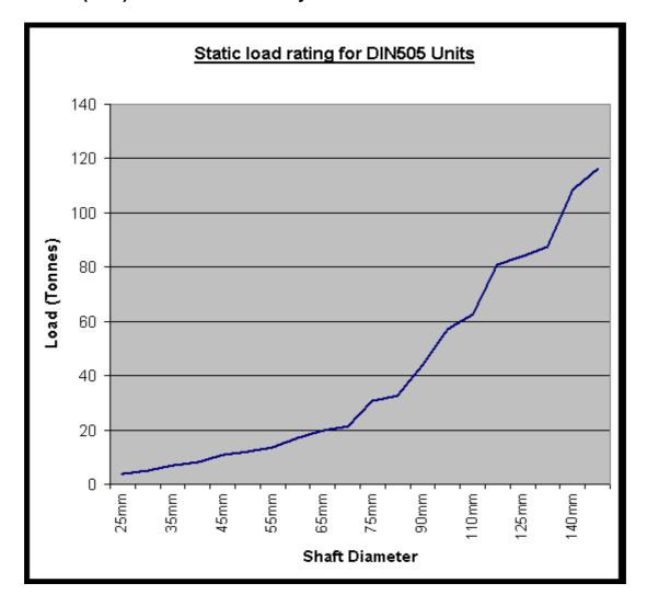
The chart shown above details the static load capacity of DIN505 units.
